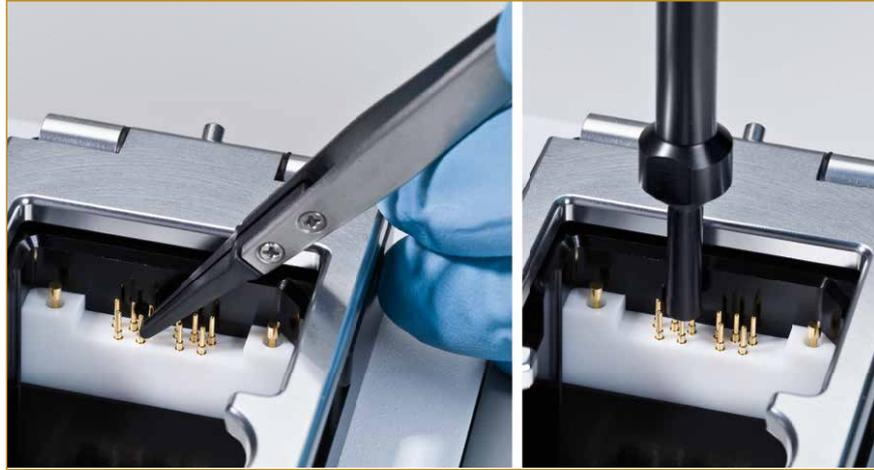
Figure 43: Replacing RTCA Contact Pins 16 (Pin GND on Cradle D3).
