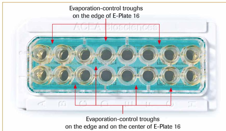
**Figure 27: Adding water in evaporation-control troughs on the edge and on the center of E-Plate 16**
