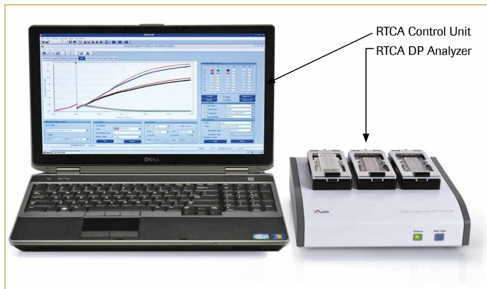
**Figure 2: The RTCA DP Instrument with the main components: RTCA DP Analyzer, and RTCA Control Unit.**
