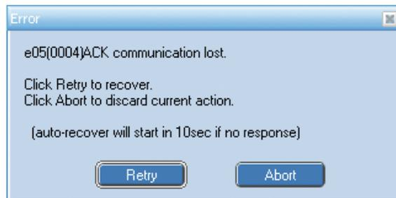
Figure 45: “ACK communication lost” error message.
