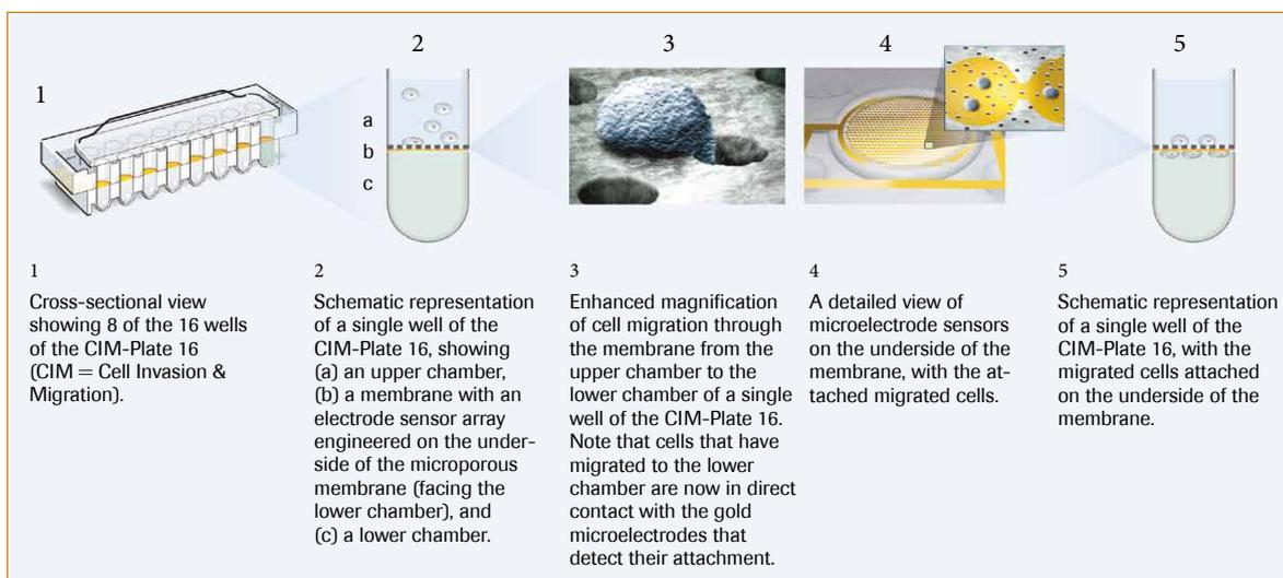
**Figure 3. Schematic illustration of the CIM-Plate 16 principle.**
