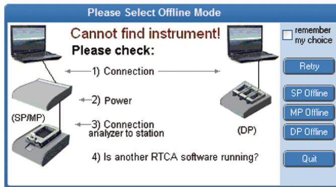
Figure 44: "Cannot find instrument" error message.
