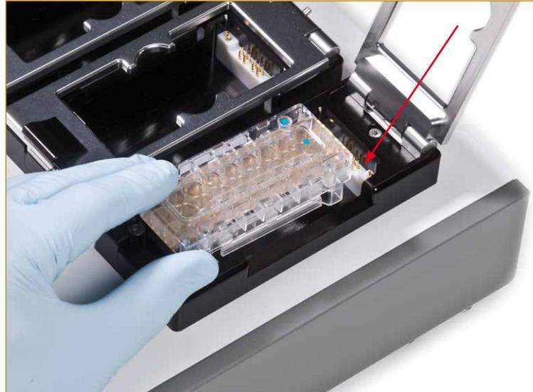
**Figure 33: Loading an CIM-Plate 16 into the D3 Cradle of the RTCA DP Analyzer (as an example).**
