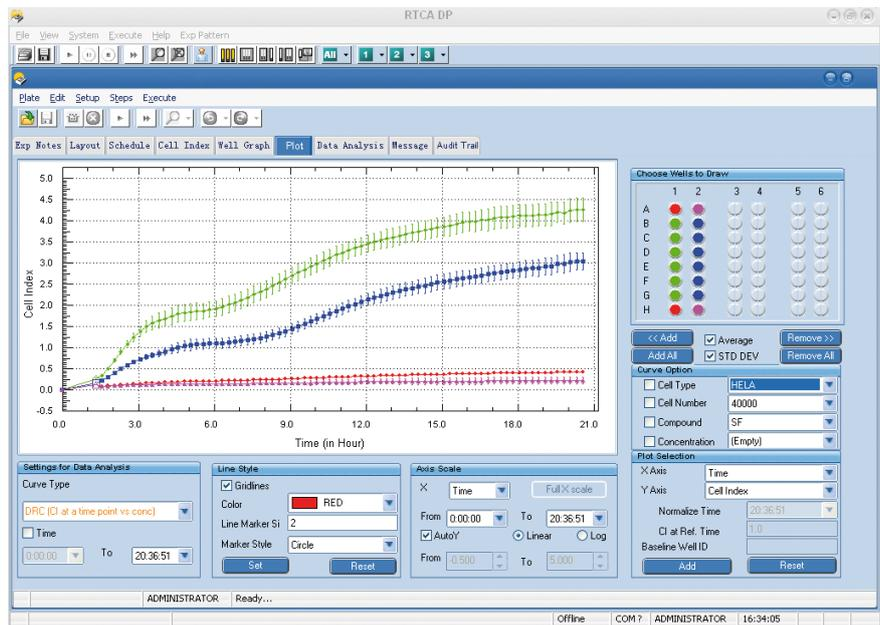
**Figure 37: Plot Page after completion of a cell migration experiment.**
