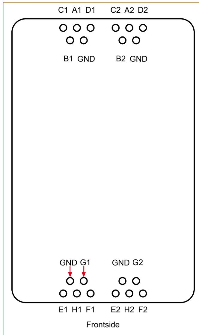
**Figure 40: RTCA Contact Pin fields. The front side of the RTCA DP Analyzer is where the LED indicator is located.**
