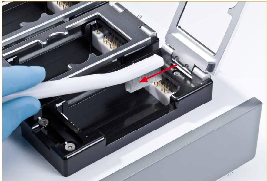
**Figure 39: Using the Nylon brush to clean the RTCA Contact Pins 16 in only one direction at a time.**
