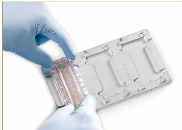
**Figure 31: Assembling the CIM-Plate 16 Upper Chamber with the Lower Chamber.**
