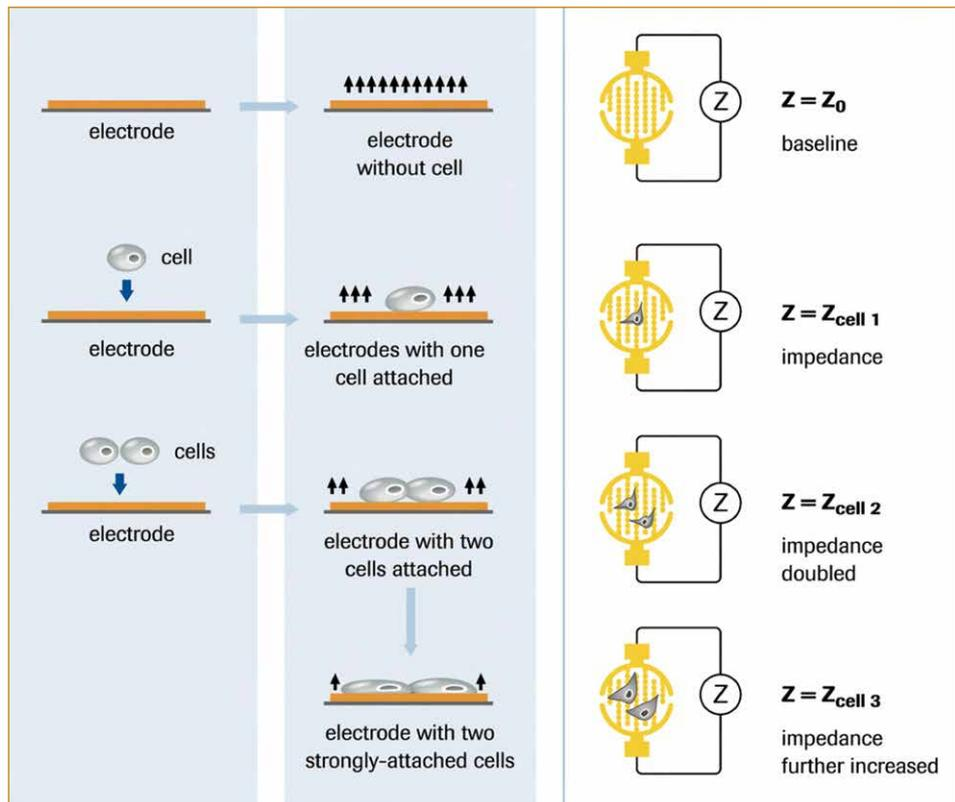
Figure 1: Schematic illustration of the impedance measurement principle.
