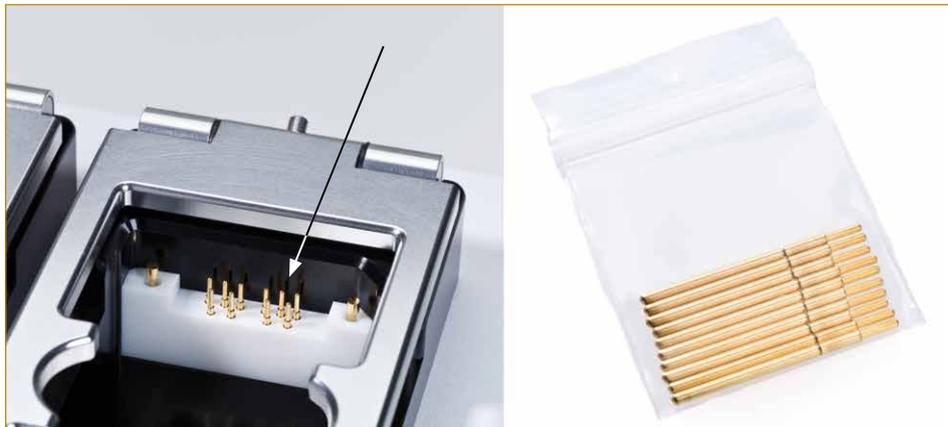
Figure 8: RTCA Contact Pins 16.
