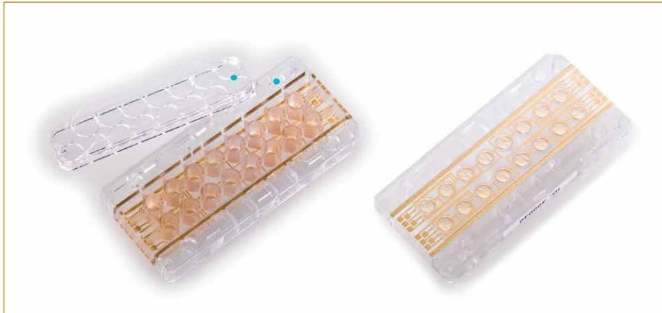
**Figure 12: Left: CIM-Plate 16 Upper Chamber with a plate cover (with blue dot in the corner of the upper chamber and middle of the plate cover). Right: Bottom side of the upper chamber.**
