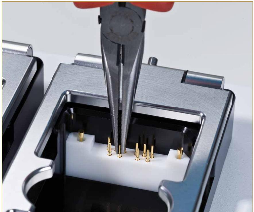
Figure 42: Extraction of an RTCA Contact Pin 16 (Pin GND on Cradle D3).
