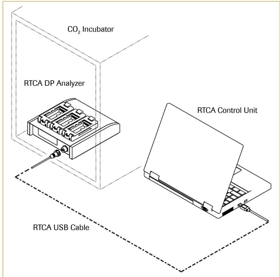
Figure 17: RTCA DP Instrument installation diagram.
