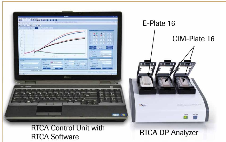
**Figure 4: The RTCA DP Instrument.**
