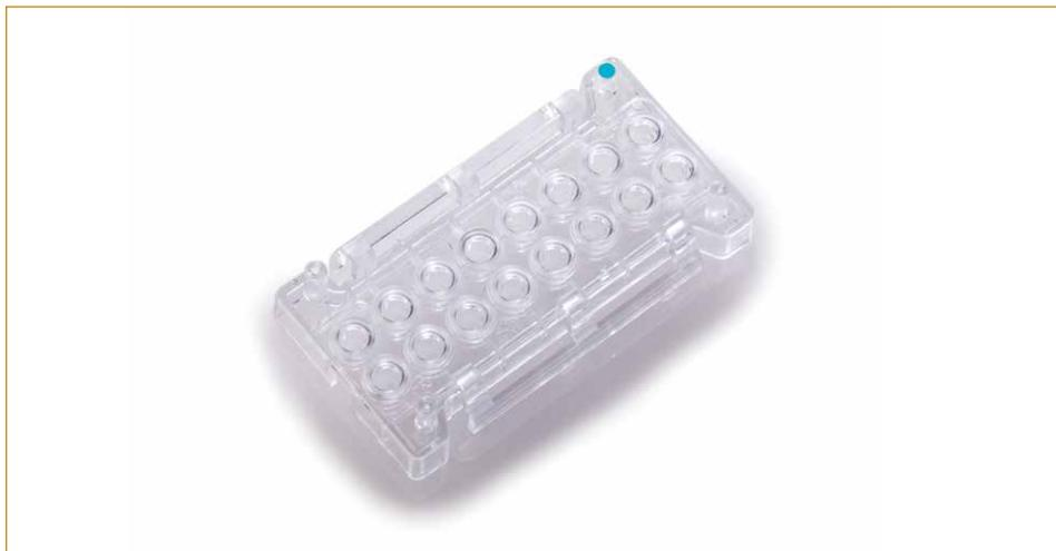
**Figure 13: CIM-Plate 16 Lower Chamber (with blue dot in the corner).**
