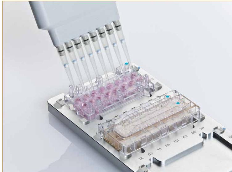
**Figure 30: Adding 160 µl media to CIM-Plate 16 Lower Chamber.**
